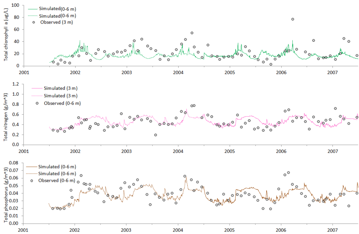
Figure 22. Comparison of model simulation results against field observations (black circles) in the surface (0 – 6 m) waters of Lake Rotorua during the calibration period (solid line) and validation period (dashed lines) for total chlorophyll a , total nitrogen and total phosphorus.
