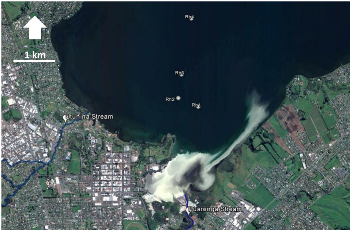
Figure 21. Satellite imagery of 17 April 2017 sourced from Google Earth illustrating the easterly dispersal of precipitated material from the geothermal area of Sulphur bay, Rotorua. Alum flocculent is discharged from the Puarenga Stream at the head of Sulphur Bay.
