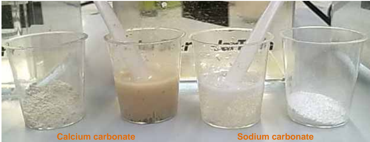
Figure 3-13 Carbonate buffer products in 62%w/v alum at low pH.
