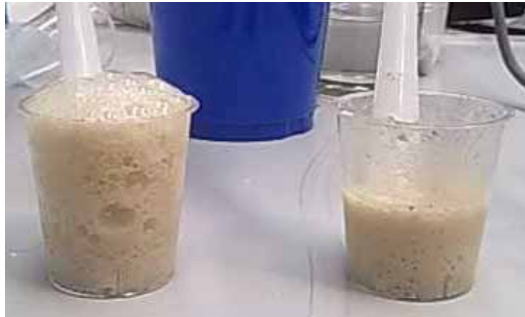
Figure 3-11 CaCO 3 in alum dissolution test
