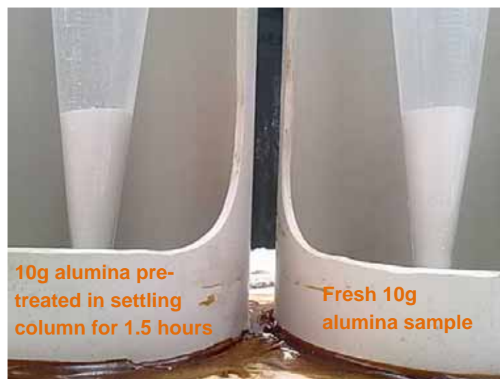
Figure 3-9 Activated alumina residuals in water
