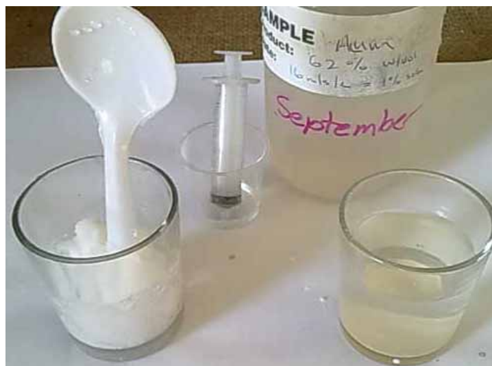
Figure 7-3 Alkali adjusted 62%w/v alum solution
