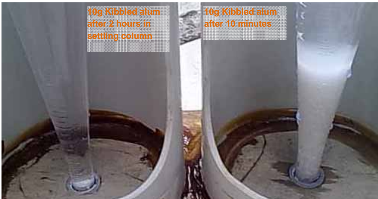
Figure 3-8 Imhoff cone measure of kibble alum solids
