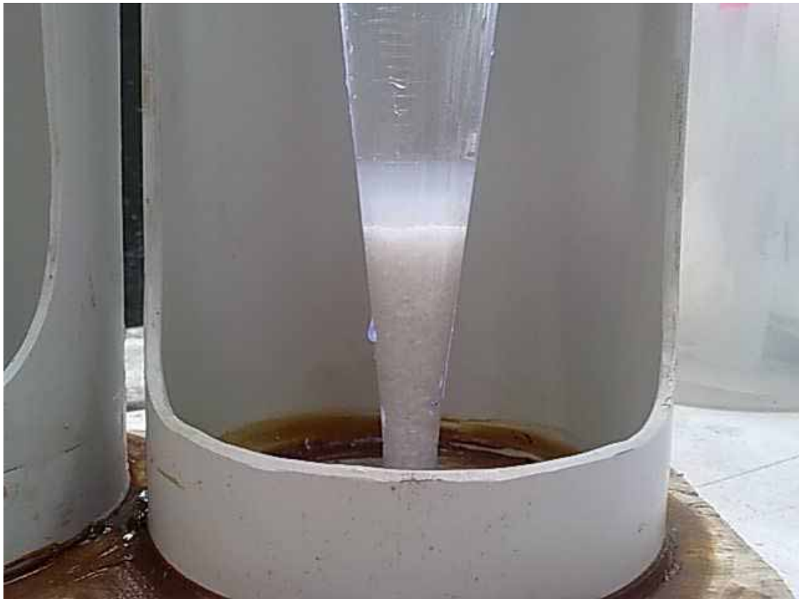
Figure 7-6 10g of kibbled alum immediately after adding to water
