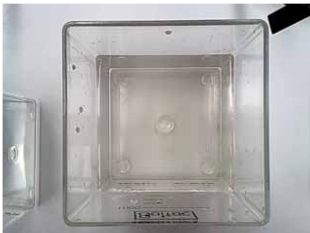
Figure 3-3 Floating floc produced by liquid alum
